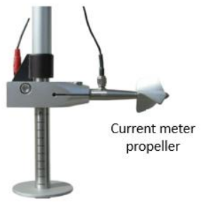
Mechanical current meter (MCM) to measure depth-averaged velocities (accuracy of ±2%)
